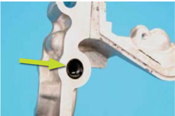
AVCS filter screens must be replaced if removed.
