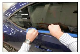
Figure 3. Example of Tape Applied to Front of Outer Door Weatherstrip
