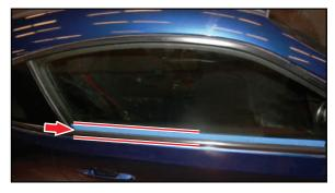
D. Apply a strip of 3M<sup>™</sup> ScotchBlue<sup>™</sup> Painter's Tape (or equivalent) vertically on the glass, parallel and adjacent to the front weatherstrip. There should be no gap between the weatherstrip and tape.
