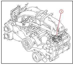
1 Fuel Pump Assembly (for High Pressure)
