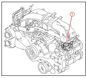
Fuel Pump Assembly (for High Pressure)
