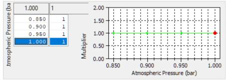
This map defines how the high and low altitude base maps are combined to produce the wastegate base duty. A value of 1.0 uses only the value from the low altitude (sealevel) base map, a value of 0.0 uses only the value from the high altitude base map. The final value for *WG Duty Base* is calculated as:
