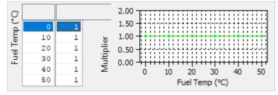
When tuning a car with a fuel temperature sensor, it is now possible to compensate for changes in the fuel temperature. Typically fuel pulsewidth is increased with increasing fuel temperature to compensate for the drop in fuel density, numbers greater than 1.0 will increase injector effective pulsewidth.
