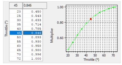
The boost target as adjusted by the **Boost Target Atmospheric Correction** map is multiplied by the output of this map. For example, a target of 2.4bar \* 0.45 = 1.08bar absolute.
