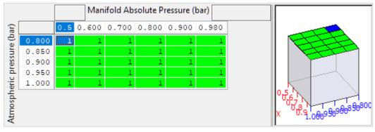
This can be used to compensate for the changes in VE typically experienced at high altitude and low atmospheric pressure. The values will multiply the VE from the SD VE map.
