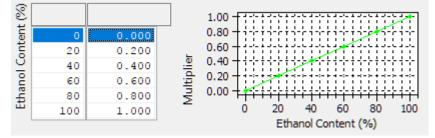
The boost limit for ethanol is blended in the same way as the boost target.
