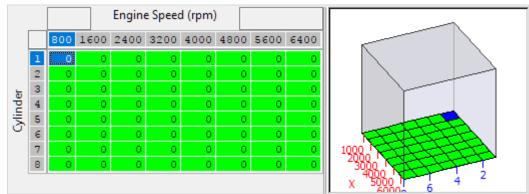
A factory map which can be used to retard the ignition on cylinders especially prone to detonation. Through careful handling and using individual cylinder knock logging, this can gain small but useful amounts of power with no increase in engine risk.
