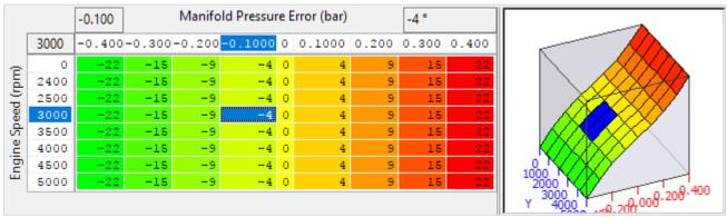
Used in conjunction with **Rolling Launch Ignition Timing Base** to deliver the **Rolling Launch Target Manifold Pressure** typically using increased retard to increase boost. The final ignition value will be capped at -30deg (30deg ATDC).
