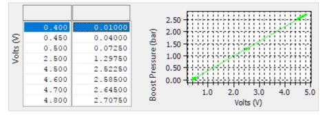
The stock scaling for the boost sensors can be replaced. However at the current time it's use is depreciated as there are some OEM strategies that use the raw voltage, resulting in odd behaviour if a pair of 4 bar sensors are used.
