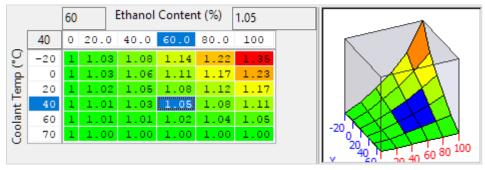
The fuel quantity at cranking will be affected by the **FlexFuel Quantity Multiplier** map however it may be required to change the fuelling further at low temperatures when cranking. This map is a 0-2 scalar and will multiply the base fuelling only when cranking.
