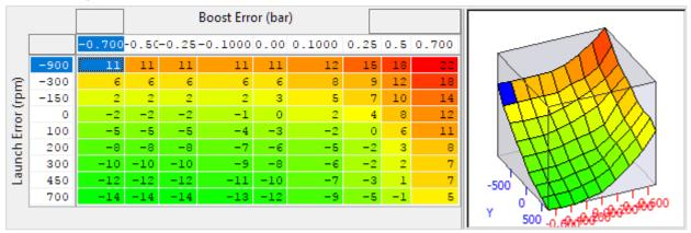
For Phase 6 the Y axis is now Launch RPM Error and allows a change in retard to help stabilise the engine speed and prevent excessive retard while the RPM is still increasing to equal the target.
