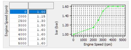
A limit of Manifold Absolute Pressure to the boost target used by the Rolling Launch antilag system. The base target is set by the values in **Rolling Launch Target Manifold Pressure** but can be reduced at specific RPM using this map. The overall target will always be the lower of the two values.
