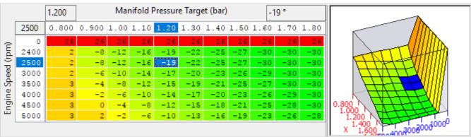
While the Rolling Launch Antilag system is active, ignition retard is used to build boost. This sets the base value, overriding the values from the main ignition maps. This map should be calibrated such that the values used are close to the final value required to make the target boost at each RPM point. Correction for boost target error comes from the **Rolling Launch Ignition Proportional** map.
