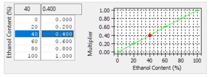
This map combines **Boost Target by Gear** and **FlexFuel Boost Target by Gear** to derive the final boost target based on *FlexFuel Ethanol content*. The eventual boost target is calculated as:
