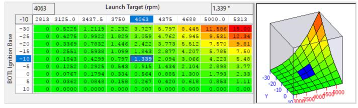
This adds an offset to the normal throttle angle depending on the current BOTL ignition retard, which is defined as the difference between the normal ignition timing as determined by the RaceROM Ignition Map for the current Mapswitch mode, and the current actual ignition timing as set by the BOTL strategy.
