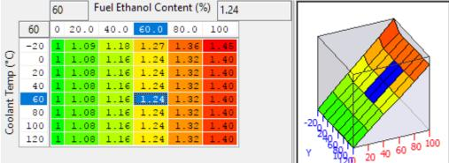
This dictates the additional fuel based on Ethanol content (0-100%) and coolant temperature. It would not be unusual to need to add additional E85 when cold due to some unburnt fuel going through the engine. Pure Ethanol typically requires 40% more fuel to maintain the same lambda (or apparent AFR) as gasoline, there is no significant change to injector flowrates when using E85.
