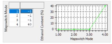
It is not always practical to add a FlexFuel sensor to every car that uses alcohol in the fuel, and many users may wish to pre-mix a specific amount of ethanol, methanol or E85 with their regular gasoline to improve performance. Premised ratios of alcohol can now be catered for in the RaceROM FlexFuel strategy but entering the ethanol content in this map.
