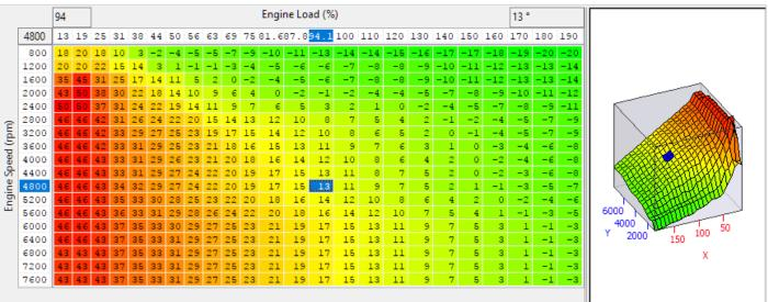
Four maps, one for each mapswitch mode providing an easy to understand and tune base ignition value in degrees BTDC. They provide increased precision and headroom for the load axis and increased RPM breakpoints. It's possible to created multiple maps and use map switching to cycle between each map for testing.
