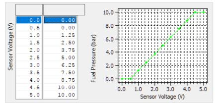
Sensor output based on input voltage.
