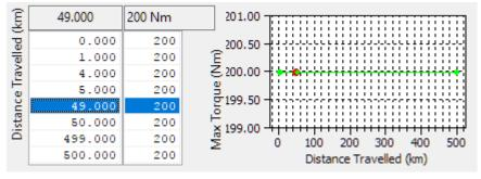
When Valet Mode is active the torque output can be limited to prevent a car being driven hard or recklessly. For use as an anti-theft measure it would be reasonable to reduce these values from the default 200Nm after a short distance.
