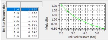
Changes in fuel pressure can be compensated for using this new map, in conjunction with an additional sensor configured using the new sensor options. For the purposes of this correction *Relative Fuel Pressure* is used and represents the pressure difference between the inlet (fuel rail) and nozzle (inlet port) pressures, defined as:
