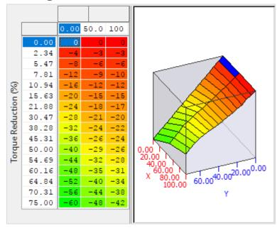
A simple lookup table that returns an ignition offset (negative values retard the ignition) to reduce the torque based on the magnitude of *CSP Torque Reduction* This map should be adjusted to allow the retard to achieve the requested torque reduction. To alter the torque reduction overall changes should be made to **CSP Torque Reduction Gain**.
