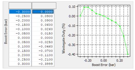
Wastegate Integral correction builds up over time. While active (see above conditions) this map dictates how much the integral value is increased with each cycle of the boost control loop. Each loop takes just 10ms (one 1/100 of a second) and the current integral correction can be observed by checking the *WG Duty Integral* live data parameter which is logged by default.
