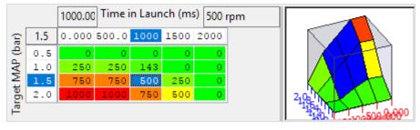
The overshoot RPM is added to the base RPM value to temporarily raise the RPM limit at the beginning of Launch Control to help the boost to be more quickly increased to the target level.
