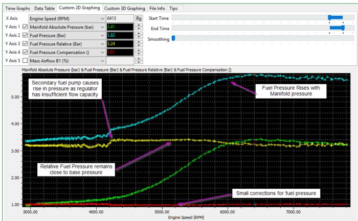
At close to sea level with an atmospheric pressure of 1.0 bar this would result in a relative fuel pressure of 3.6 bar if the Gauge Fuel Pressure was 4.9 bar at 2.3 bar MAP (1.3 bar relative boost).
