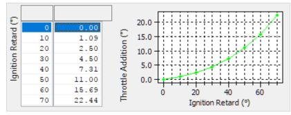
This map adjusts the throttles to compensate for torque variations as the ECU varies the ignition timing to generate boost. The compensation is now an absolute throttle angle adder and the above table has shown to give sensible results but may need fine tuning.
