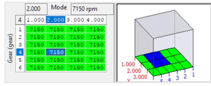
To simplify the setting of the fuel cut based rev limits, they now all appear in one 3d map and use a single 1d value to introduce hysteresis. The fuel cut will be active over the RPM value in this map, and fuel will only be restored when the RPM has dropped below this level by **Rev Limit Hysteresis**.
