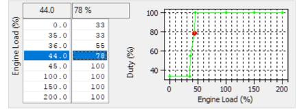
Direct fuel pump control is ONLY ENABLED WHEN 12 INJECTOR CONTROL IS ENABLED! So if you wish to use these maps, enable 12 injector control in all your map switch modes and set the enable RPM to 10000rpm so that it never comes on. Remember when 12 Injector Support is enabled the secondary air solenoid output will be hijacked.
