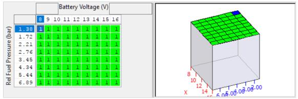
The OEM injector lag time (latency) is defined using a fixed voltage and a slope that gives accurate lag time over a narrow voltage range. It's of limited accuracy, not very intuitive to set up and injector suppliers rarely give useable data for both lag time *and* slope. Instead, RaceROM now provides a 3D map using voltage and fuel pressure to allow complete control of the lag time.
