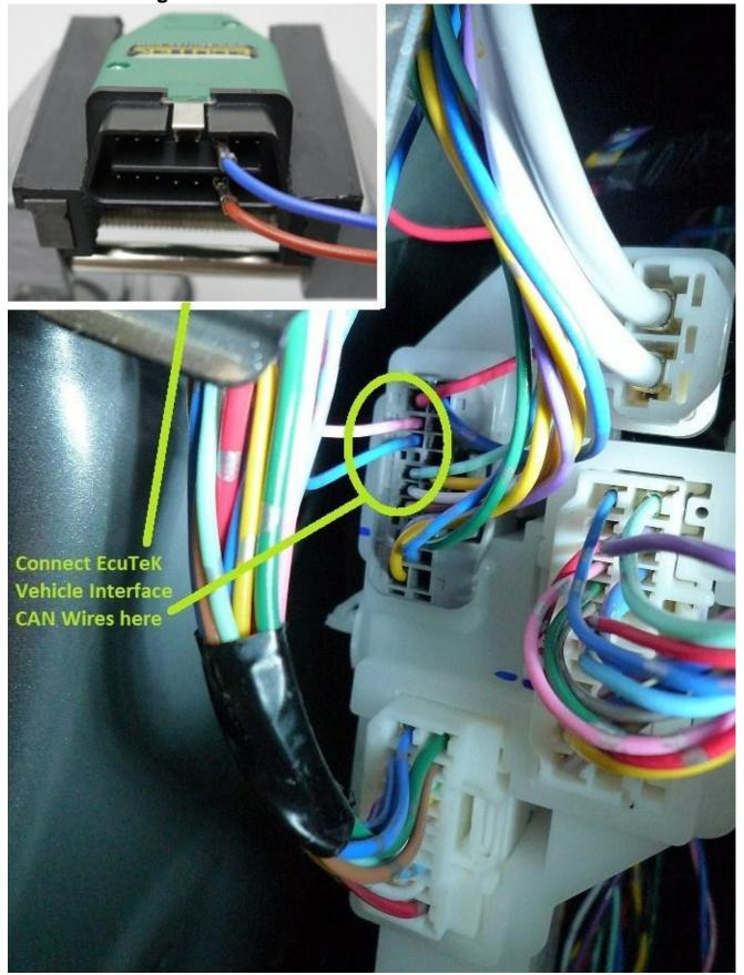
The above picture shows the actual **C-128** connector on a 2012 ASX model. Please note that the wire colours could be different on another Mitsubishi model.
