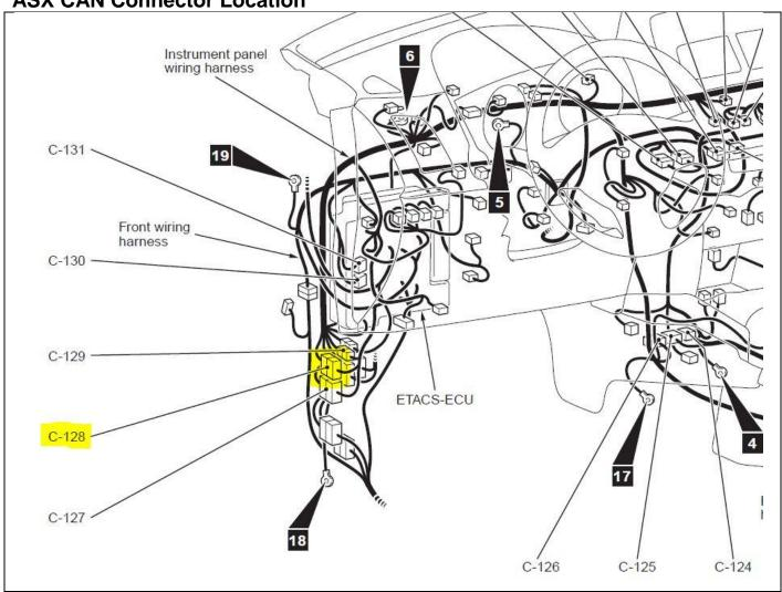
The above image shows the **C-128** connector that the EcuTek Vehicle Interface cable needs to be connected to.
