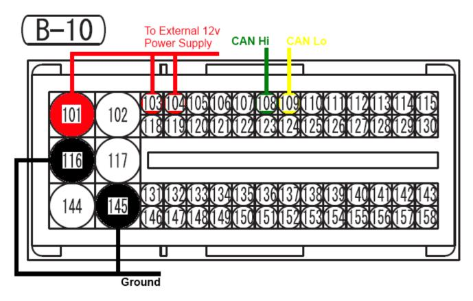
The wires will have to connect directly to the ECU pins, so please make sure the crimp terminals are well insulated and do not short against other exposed pins. This may cause damage to your ECU. We suggest using a small length of heat shrink tube to insulate any bare metal of the terminal.
