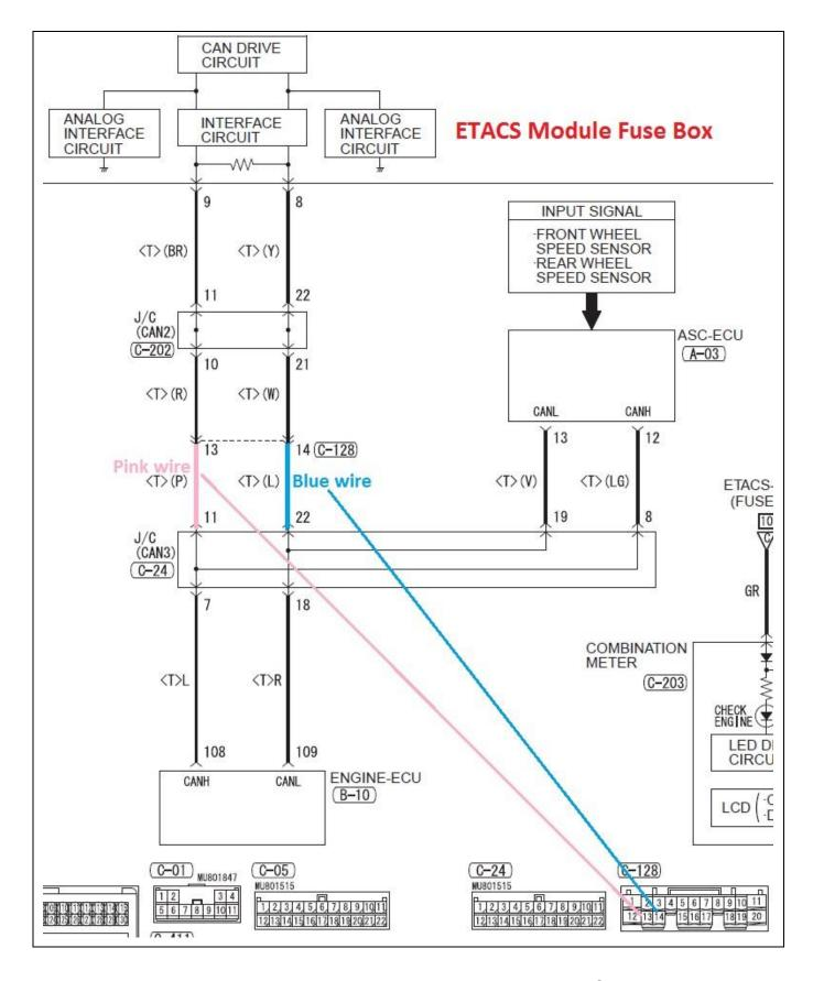
This image shows that we need to connect to pin 13 and pin 14 on the C-128 connector.
